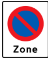
E68: Zone with no parking
