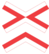
A74.2: Cross-mark for multi track railway crossing
