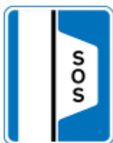
E34: Emergency bay
