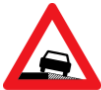
A35: Dangerous verge
